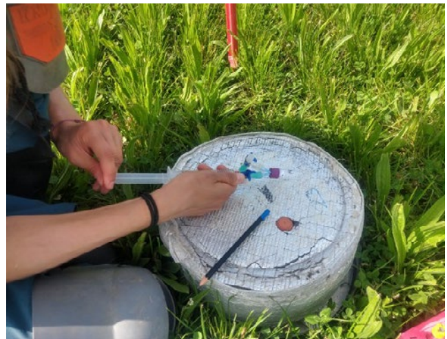
Measuring nitrous oxide emissions in the field with a lysimeter https://www.nzagrc.org.nz/domestic/nitrous-oxide-research-programme/plants-and-nitrous-oxide-emissions/
